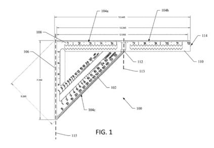
Ex. A, Fig. 1. The inventions described and claimed in these patents are valuable. For example, the extension element allows a craftsman to use the same size speed square for multiple different size materials. The craftsman can retract the extension element when working with smaller materials and extend it when working with larger materials.
