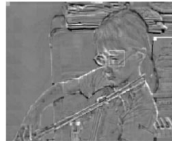
Figure 6.8 Residual after subtracting intra prediction
