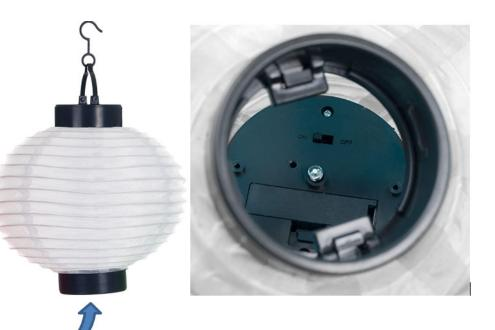
15. The accused TMG Collapsible Lanterns include a lighting element assembly with an LED light serving as a lighting element. As shown in the interior view above at the right, the LED extends below the lighting element assembly and into the collapsible shade. A housing receives a solar cell and battery. The collapsible shade is attached to the housing and supported by a collapsible wire frame.
