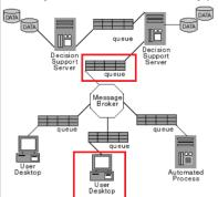
29. On information and belief, the Accused Instrumentality practices detecting a producer worker (e.g., producer application) at a first server (e.g. SAS server), wherein the producer worker (e.g., producer application) sends a first message to a datacenter queue (e.g. SAS message queue) at least partially stored at a second server (e.g. Message Queue server).
