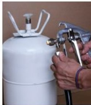
4: Attach standard gun to large end of hose. Hand tighten, using a 3/4" wrench to fully tighten.
