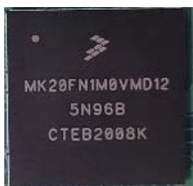
Images of the Freestyle Libre 2 processors in the sensor and handheld receiver.
