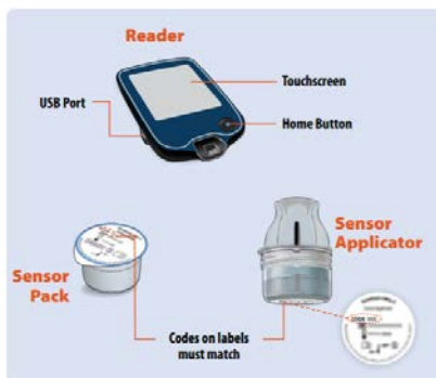
Images of the Freestyle Libre 2 processors in the sensor and handheld receiver.
