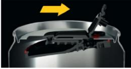
24. The sealing element itself is fixedly connected to the cover of the can in the area opposite the opening, which itself creates a bias of the sealing element in relation to the cover with
