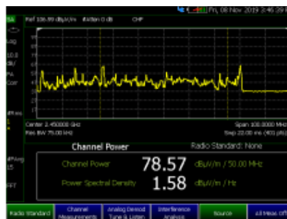
EMF measurement using spectrum analyzer channel power mode
