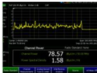
EMF measurement using spectrum analyzer channel power mode
