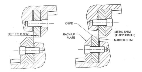
24. On information and belief, the element labeled as a "BACK-UP PLATE" is a clamping block as recited in the claims of the '271 patent.
