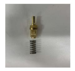
29. The HK Army regulator has pin valve positioned in the piston bore.
