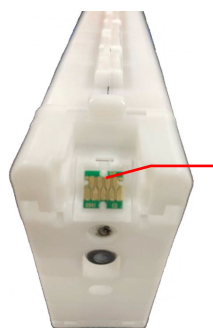
printed circuit board (green) with low voltage electronic device located on back
