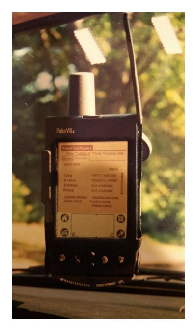
57. The prototype was constructed using a Palm VIIx personal digital assistant combined with a GPS clip from a different manufacturer, and new software written to connect the assembled hardware components and communicate with a remote real estate database. The inventors of the Patents-in-Suit thus anticipated the use of a customized software application on a GPS-enabled mobile device for real estate searching several years before the advent of smartphone apps.
