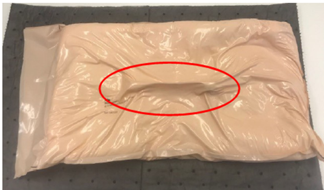
Figure 5. Positioner created without vacuum after the pinch test showing a looser, non-snug fit over the inner beads
