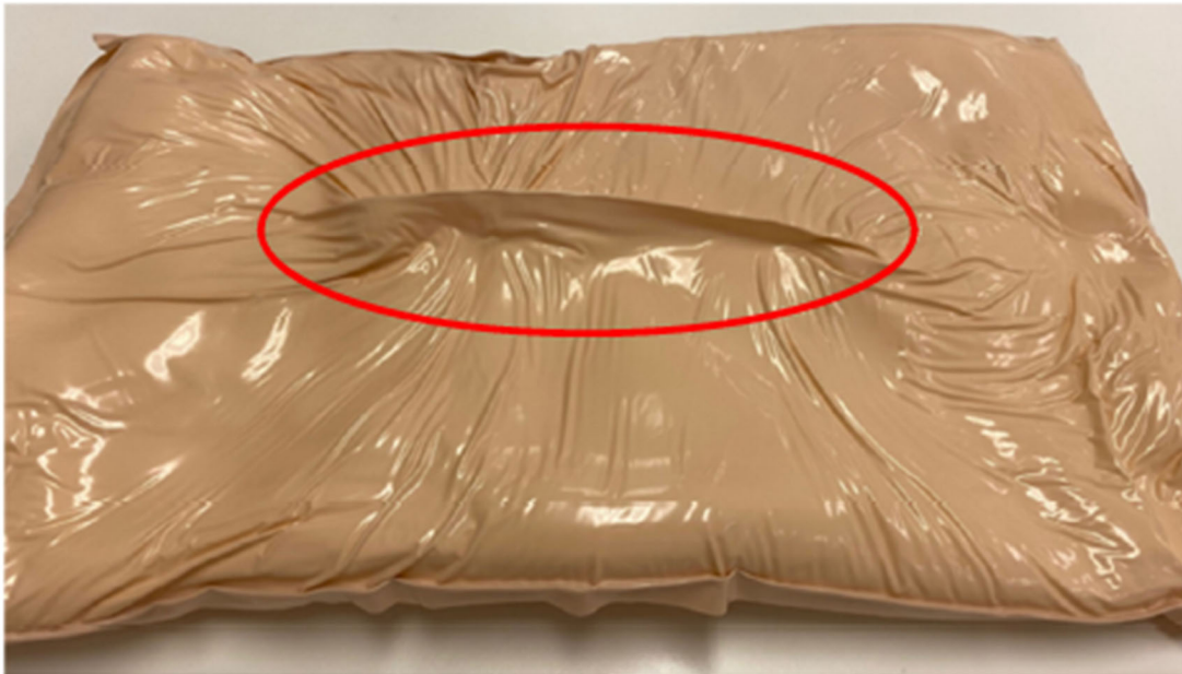
Figure 3. MHC's positioner after the pinch test showing a tight, snug fit around the inner beads
