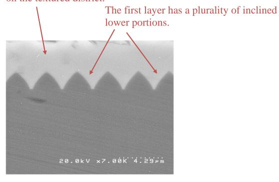
19. The LEDs used in the Accused Products use a gallium nitride first layer.
