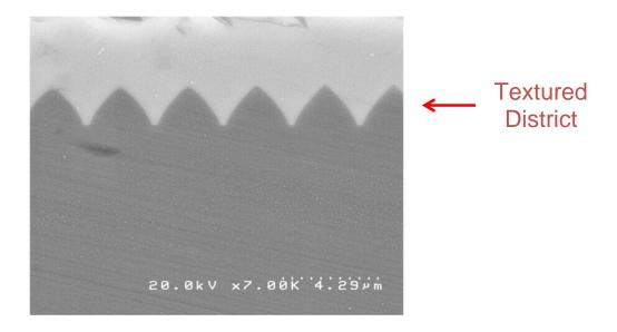
The plurality of etched trenches has sloped etching profiles with a smooth rotation of micro-facets without a prescribed angle of inclination.
