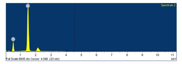
The substrate is comprised of sapphire (Al<sub>2</sub>O<sub>3</sub>).
