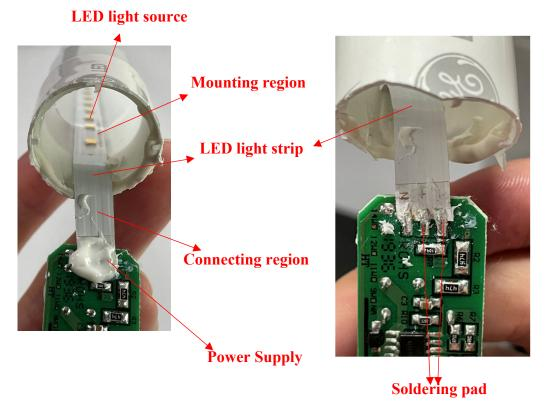
59. The LED14BDT8/G4/840 further comprises a protective layer disposed on a surface of the LED light strip, the protective layer having a plurality of first openings to accommodate the plurality of LED light sources and at least two second openings to accommodate the at least two soldering pads:
