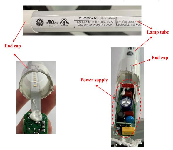
68. The LED14BDT8/G4/840 further comprises an LED light strip attached to an inner circumferential surface of the glass tube and a plurality of LED light sources mounted on the LED light strip:
