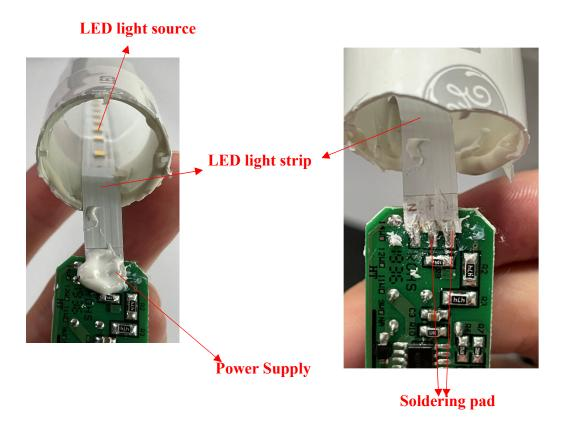
69. The LED14BDT8/G4/840 further comprises at least two first soldering pads arranged at one end of the LED light strip and a protective layer disposed on a surface of the LED light strip, the protective layer comprising at least two first opening to expose the two first soldering pads:
