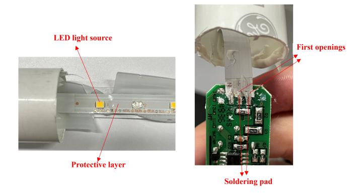
70. The LED14BDT8/G4/840 further comprises a power supply module comprising a printed circuit board and configured to drive the plurality of LED light sources, the printed
