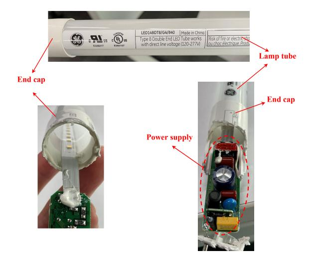
58. The LED14BDT8/G4/840 further comprises an LED light strip disposed on an inner circumferential surface of the lamp tube, the LED light strip comprising a mounting region and a connecting region, the mounting region for mounting a plurality of LED light sources, the connecting region having at least two soldering pads, and the mounting region and the connecting region being electrically connected to the plurality of LED light sources and the power supply:
