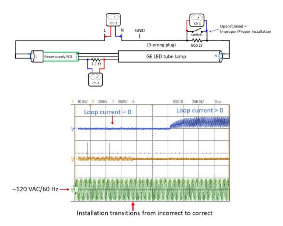
48. The signal generated from the external driving signal on the LED14BDT8/G4/840 is a sampling signal on the power loop, the installation detection circuit further comprises a detection determining circuit configured to detect the sampling signal for determining whether the LED tube lamp is properly installed on the lamp socket, and the power loop includes the switch circuit and the detection determining circuit:
