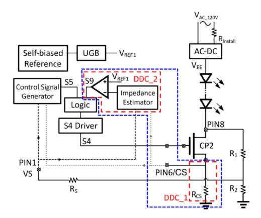
80. When the signal level of the transient current is smaller than the predefined signal, the installation detection module limits a current on the power loop to less than 5 MIU (measurement indication units) by controlling a conduction state of the power loop, by opening a switch CP2 on the power loop. For example, when the LED tube lamp is improperly installed, the loop current remains below 5 MIU:
