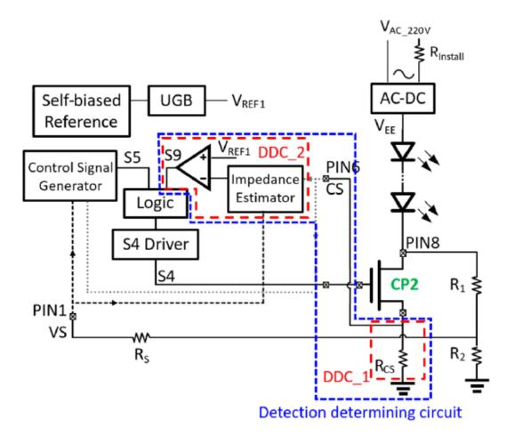
49. The installation detection circuit in the LED14BDT8/G4/840 further includes a detection result latching circuit coupled to the switch circuit, wherein the detection result latching circuit is configured to receive the one or more pulse signals to control turning on and off of the switch circuit based on a detection result signal from the detection determining circuit:
