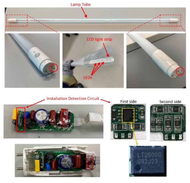
44. The installation detection circuit comprises a pulse generating circuit configured to output one or more pulse signal. For example, a simplified circuit diagram based on a
