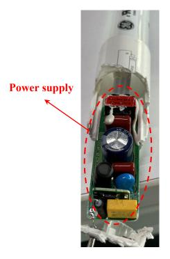
71. The power supply module comprises a rectifying circuit and a filtering circuit coupled to the rectifying circuit:
