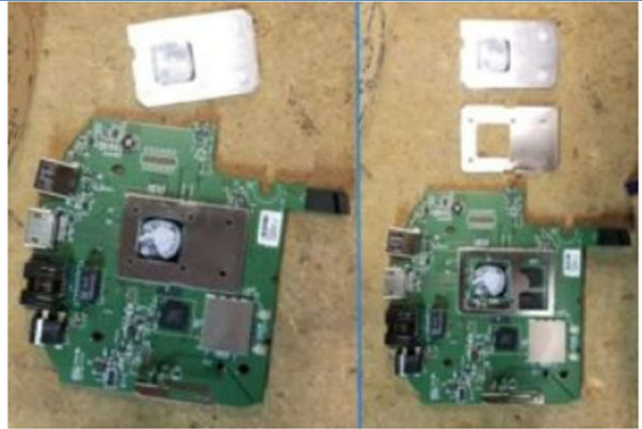
The two-piece heat sink in stages of disassembly. Click image to enlarge.
