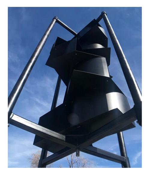
25. The Infringing Product includes each of the lips being configured for reducing three-dimensional aerodynamic effects on the turbine, and defined as a horizontal structure substantially corresponding to the curvature of the trailing portion of the at least one curved blade.
