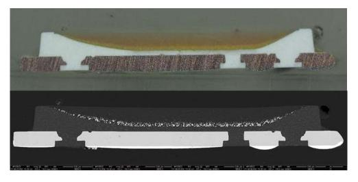
140. Also shown in the image above is an encapsulating molding part formed over and around the light-emitting diode chip. The molding part is a silicon based encapsulant. The relatively
