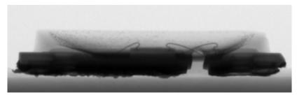
123. The image at bottom shows a SEM image of a cross-section through the package. The image shows the resin member contains phosphor particles, which can be seen as relatively bright spots within the darker resin.
