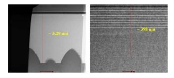
109. Below are two Scanning Electron Microscope (SEM) images of an LED chip from the Finelite HPR-A-2X2-S-835-DCO-LED-3500K-277V-SC-C1-OBO LED panel. The image on the left shows the p-pad, with three conductors extending from the p-pad. The image on the right was created after the creation of a hole in the LED using a focused ion beam (FIB).
