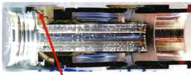
resilient electrically-conductive grounding member between the post and the coupler and contacting both
