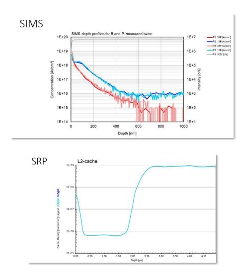
106. The Intel Core i7 11800H contains at least one well region adjacent to the first or second active region containing at least one graded dopant region, the graded dopant region to aid carrier movement from the surface towards the area of the substrate where there are no active regions, wherein at least some of the transistors form digital logic of the VLSI semiconductor device.
