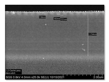
70. The Intel Core i7 11800H has an active region including a source and a drain, disposed on one surface of said surface layer.
