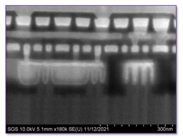
83. The Intel Core i7 11800H has at least a portion of at least one of the first and second active regions having at least one graded dopant concentration to aid carrier movement from the first surface to the second surface of the substrate.
