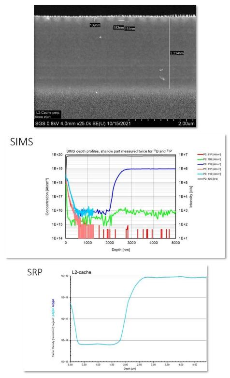
80. The Intel Core i7 11800H has a first active region disposed adjacent the first surface of the substrate with a second doping type opposite in conductivity to the first doping type and within which transistors can be formed. See images below.
