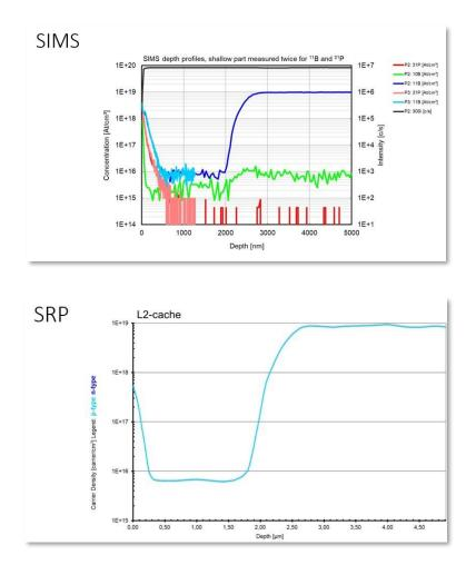
103. The Intel Core i7 11800H contains a first active region disposed adjacent the surface with a second doping type opposite in conductivity to the first doping type and within which transistors can be formed.
