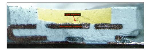
*I(d): a transparent sealing resin that seals the light emitter, and forms a concave surface that is a light-outgoing surface via which light outgoes,*— The Ikea Molgan and the Ikea Dioder LED light each comprises a transparent sealing resin that seals the light emitter, and forms a concave surface that is a light-outgoing surface via which light outgoes.
