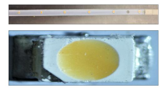
*1(b): a placement surface that includes an electrode;* — The Ikea Molgan and the Ikea Dioder LED light comprises a placement surface that includes an electrode.
