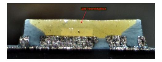
As another example, shown below is the cross-sectional view of the LED from the Ikea Ledare 5.5W E26 LED Bulb with the light transmitting resin formed on the light emitting element and first and second lead frames identified:
