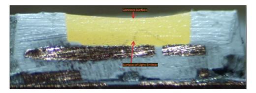
As another example, shown below is a cross-sectional view of the LED from the Ikea Dioder LED light with the concave surface facing a surface of the light emitter identified:
