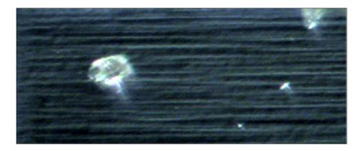
As another example, a face of the reflector formed into a rough surface is shown in the below image of a Ikea Ryet G4's reflector:
