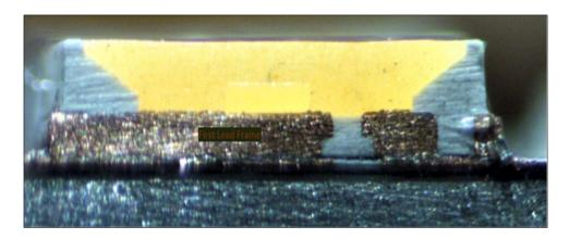
As another example, shown below is a resulting cross-sectional view of one crosssectioned LED chip from the Ikea Ryet 1717G5 LED Bulb with a first lead frame having a main surface on which the light-emitting element is mounted identified:
