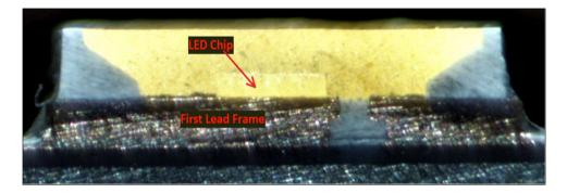
As another example, shown below is a resulting cross-sectional view of the one crosssectioned LED chip from the Ikea Ryet E12 LED Bulb with the one cross-sectioned LED chip mounted to a first lead frame identified:
