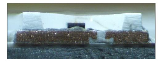
As another example, and in more detail, shown below is a scanning electron microscope ("SEM") image showing a reflective layer formed on a support substrate from the Ikea Tradfri E26 LED Bulb. As shown, the substrate is a ceramic material, and a reflective layer is formed on the substrate:
