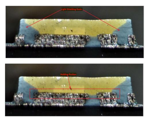
As another example, shown below is the cross-sectional view of the LED from the Ikea Ledare 5.5W E26 LED Bulb with the light shielding resin and holding portion identified:
