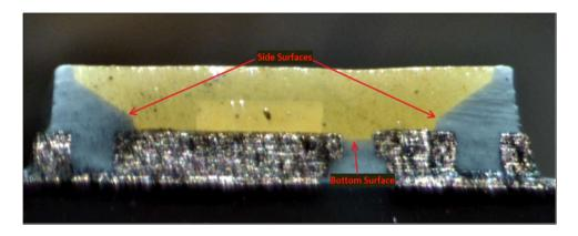
As another example, shown below is the cross-sectional view of the LED from the Ikea Ledare 5.5W E26 LED Bulb with the light shielding resin covering a bottom surface and a side surface of the holding portion identified:
