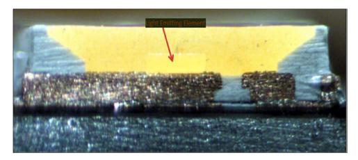
As another example, shown below is a cross-sectional view of the LED from the Ikea Ryet 1717G5 LED Bulb with the light-emitting element identified:
