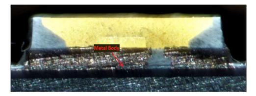
As another example, this configuration is shown in the below cross-sectional view of a cross-sectioned LED chip from the Ikea Ryet E12 LED Bulb:
