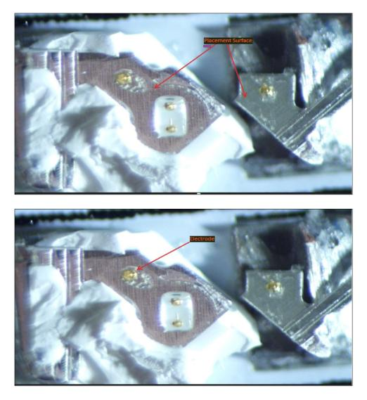
As another example, shown below are top down views of an LED from the Ikea Dioder LED light with a placement surface that includes an electrode identified:
