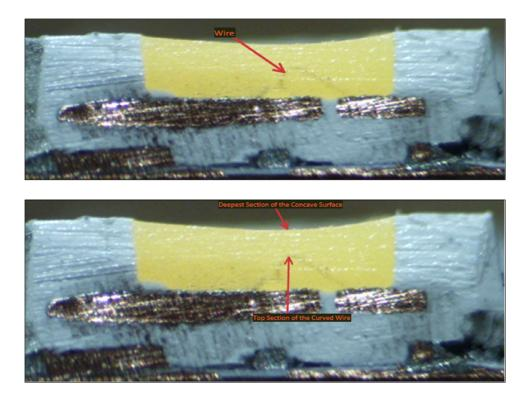
As another example, shown below is a cross sectional view of the LED from the Ikea Dioder LED light with the light emitter and the electrode connected via a wire that is curved in such a way that a top section of the curved wire substantially coincides with a deepest section of the concave surface:
