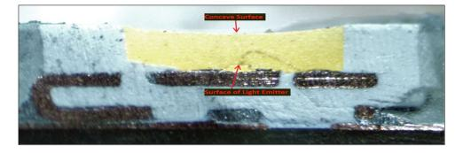
1(f): the light emitter and the electrode being connected via a wire that is curved in such a way that a top section of the curved wire substantially coincides with a deepest section of the concave surface,— The Ikea Molgan and the Ikea Dioder LED light each includes a light emitter and the electrode being connected via a wire that is curved in such a way that a top section of the curved wire substantially coincides with a deepest section.
