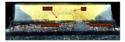
As another example, shown below are cross-sectional views of the cross-sectioned LED chip from the Ikea Ryet E12 LED Bulb with a second lead frame electrically connected to the LED chip via a wire identified:
