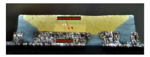
As another example, shown below is a resulting cross-sectional view of one crosssectioned LED chip from the Ikea Ledare 5.5W E26 LED Bulb with a first lead frame having a main surface on which the light-emitting element is mounted:
