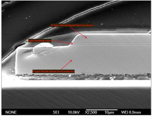
As another example, shown below is a close-up SEM image of the cross-sectioned LED chip from the Ikea Tradfri E26 LED Bulb identifying a p-type nitride-based semiconductor layer,
