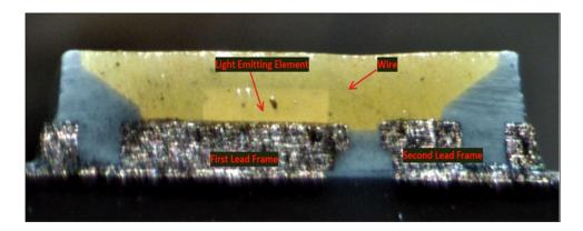
As another example, shown below are cross-sectional views of the phosphor LED chip from the Ikea Ledare 5.5W E26 LED Bulb with the second lead frame electrically connected to the semiconductor light emitting element via a wire identified:
