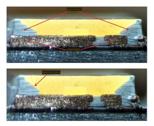
As another example, shown below is a cross-sectional view of the phosphor LED chip from the Ikea Ryet 1717G5 LED Bulb showing the resin portion for fixing the first lead frame, and the reflecting portion reflecting light from the light-emitting element:
