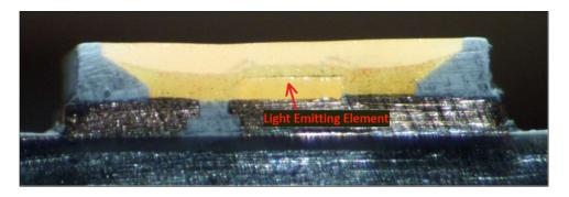
As another example, shown below is the cross-sectional view of the example phosphor LED from the Ikea Ryet G4 with the light emitting element on the substrate identified:
