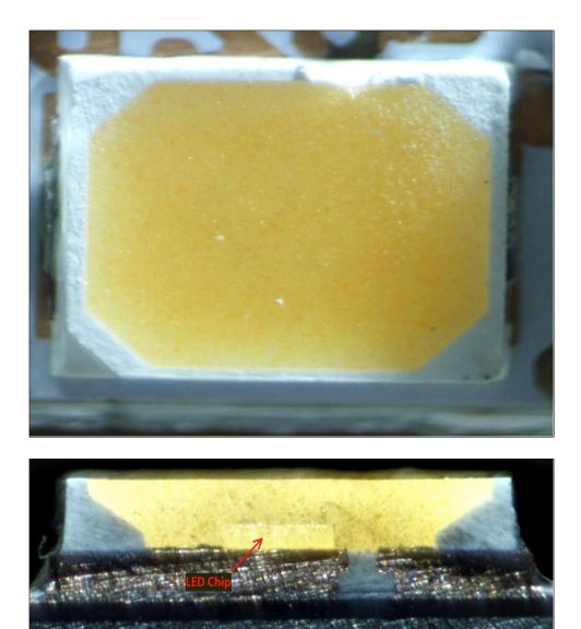
As another example, shown below are a top-down view and a cross-sectional view of the phosphor LED from the Ikea Ryet E12 LED Bulb, respectively:
