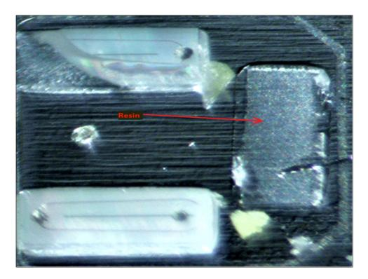
As another example, shown below is a top-down view of the example LED from the Ikea Ryet G4 with the LED removed and the resin disposed between the light emitting element identified:
