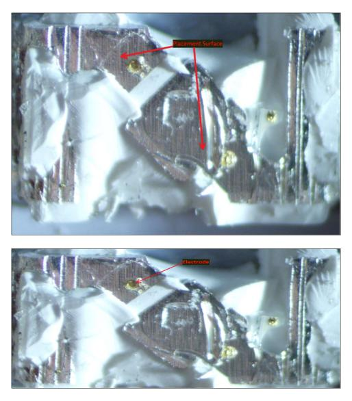
*1(c): a light emitter that is placed on the placement surface;*— The Ikea Molgan and the Ikea Dioder LED light comprises a light emitter that is placed on the placement surface.
