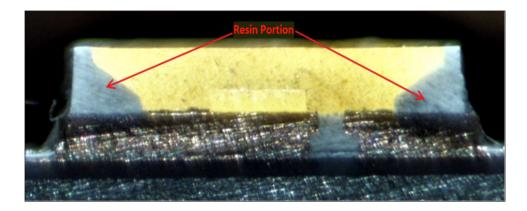
As another example, shown below is a cross-sectional view of a LED chip from an Ikea Ryet E12 LED Bulb with a resin portion surrounding the circumference of the LED chip and fastening first and second lead frames identified:
