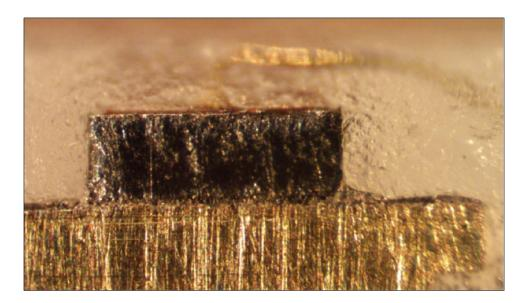
As another example, and in more detail, shown below is a scanning electron microscope ("SEM") image showing a reflective layer formed on a support substrate from the Ikea LEDberg Multicolor Lightstrip. As shown, the substrate is a ceramic material, and a reflective layer is formed on the substrate:
