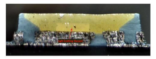
As another example, a cross section of an LED from a Ikea Ledare 5.5W E26 LED Bulb was taken, and a resulting cross-sectional view is shown below with a semiconductor light emitting element identified:
