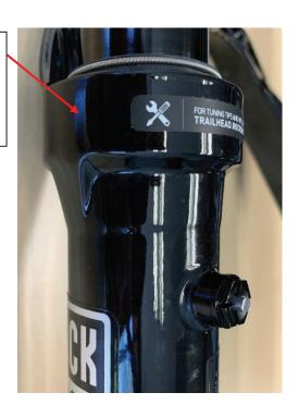
25. SRAM's RockShox Lyrik Ultimate includes an air bleed assembly disposed on said lower leg fork tube, said air bleed assembly configured for equalizing ambient pressure within said lower fork tube, as illustrated in the exemplary photographs of SRAM's RockShox Lyrik Ultimate.
