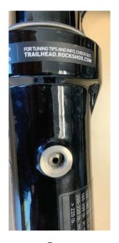
26. Said air bleed assembly of SRAM's RockShox Lyrik Ultimate includes a fluid passage disposed between an interior of said lower fork tube and an exterior of said lower fork tube, as illustrated in the above exemplary photo of the Rock Shox Lyrik Ultimate fork.
