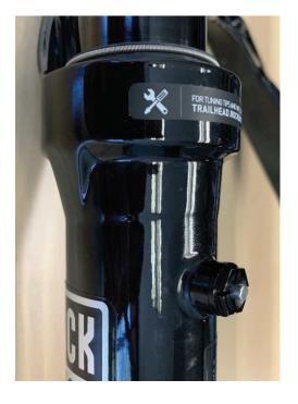
28. Said manually operable valve of SRAM's RockShox Lyrik Ultimate has a second position allowing a fluid to flow between said interior and said exterior, as illustrated in the exemplary photo of the Rock Shox Lyrik Ultimate fork.
