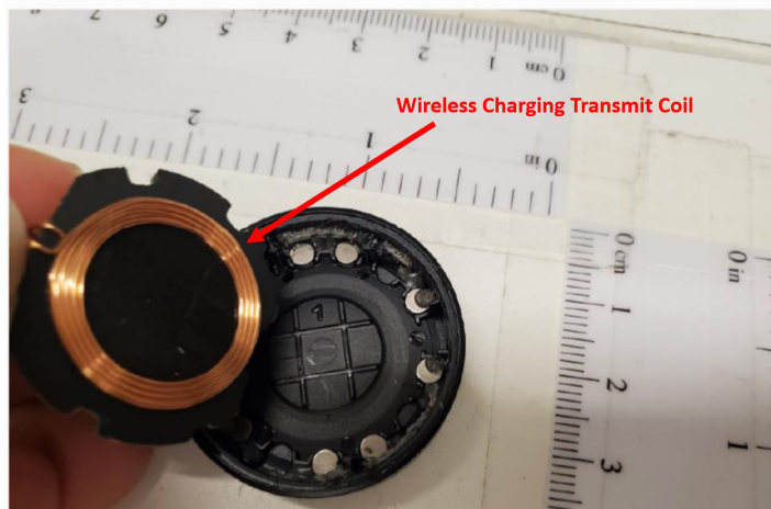
(FCC MASIW1CG Masimo W1 Charger Internal Photos (annotation added)). 40
