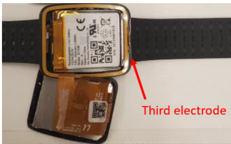
(FCC MASIW1 Internal Photos (annotations added)).
