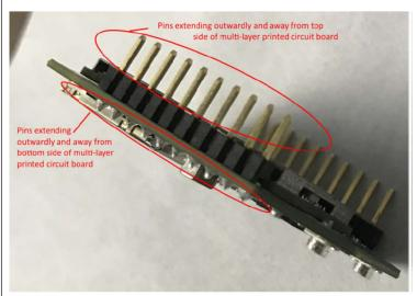
a second plurality of electrically conductive pins in electrical connection with the cellular transceiver module and aligned along a second pin axis to form a second row of pins, each of the second row of pins extending outwardly and away from the bottom side of the multi-layer printed circuit board, the second row of pins located opposite the first row of pins; and
