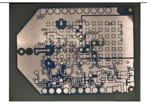
The Digi XBee Cellular Modem includes a second layer including a ground plane. The second layer is labeled "Layer 2" in the side-view photo above and is shown below:
