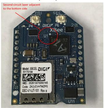
A ground plane layer is between the first and second layers:
