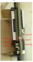
The Digi XBee Cellular Modem includes a first layer having one or more circuits. The first layer is labeled "Layer 1" in the side-view photo above and has one or more circuits:
