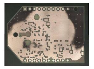
The Digi XBee Cellular Modem includes a third layer including a power plane. The third layer is labeled "Layer 3" in the side-view photo above and is show below:
