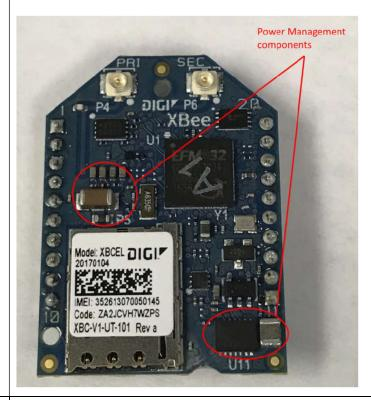
a first plurality of electrically conductive pins in electrical connection with the cellular The Digi XBee Cellular Modem has a first plurality of electrically conductive pins in electrical connection with the cellular transceiver module and aligned
