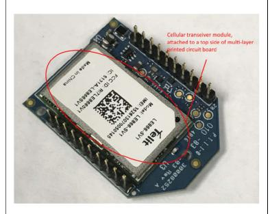
electrical power-management components attached to the multi-layer printed circuit board, the power-management components in electrical communication with the cellular transceiver module; The Digi XBee Cellular Modem has electrical power-management components attached to the multi-layer printed circuit board. The power-management components are in electrical communication with the cellular transceiver module:
