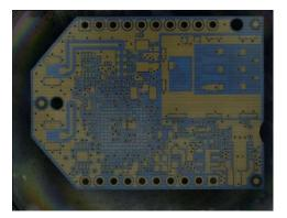
The first layer of the Digi XBee Cellular Modem is soldermasked to form the first side of the multi-layer printed circuit board. As shown above, the first layer is "Layer 1" and forms the first side of the PCB.
