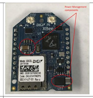
a first plurality of electricallyconductive pins aligned along a first pin axis to form a first row of pins, each of the first plurality of pins extending outwardly and away from the multi-layer printed circuit board, one or more of the first plurality of electricallyconductive pins in electrical connection with the cellular transceiver module and one or more of the first plurality of electrically-conductive pins in electrical connection with the electrical power-management components;
