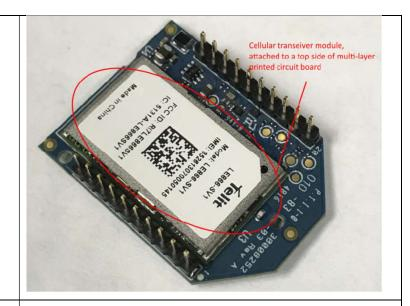
electrical power-management components attached to the multilayer printed circuit board, the power-management components in electrical communication with the cellular transceiver module; The Digi XBee Cellular Modem has electrical power management components attached to the multi-layer printed circuit board and in electrical communication with the cellular transceiver module:
