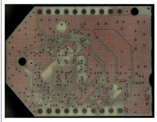
a cellular transceiver module configured to communicate over a cellular wireless cellular network, the cellular transceiver module comprising a processor and attached to a top side of the multi-layer printed circuit board; The Digi XBee Cellular Modem has a cellular transceiver module with a processor attached to the top side of the multi-layer printed circuit board:
