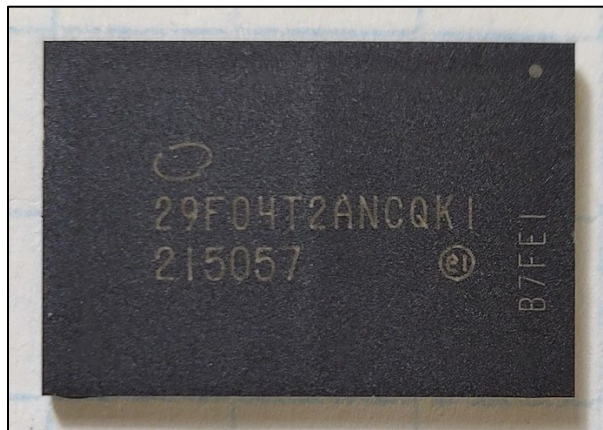
3D NAND Chip (29F04T2ANCQKI) Extracted from Intel's SSD 670p Series
