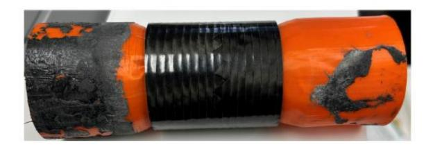
38. The spacer appears to be made of plastic-like material and it may include air gaps or bubbles between layers thereby having the structure of foam.
