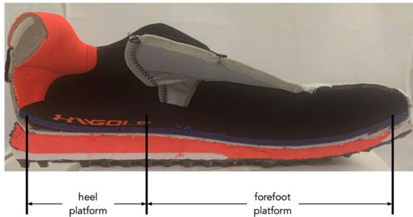
Figure 27. Cross-cut of the HOVR Forge RC Spikeless shoe, showing the heel and forefoot platforms.
