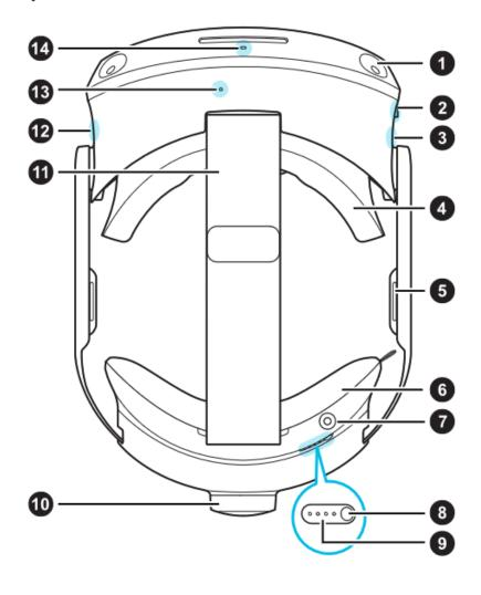
1 Headset camera (4x) 2 3.5mm audio jack 3 USB Type-C® port 4 Face cushion and frame 5 Built-in speaker 6 Back pad 7 Charging port 8 Power button 9 Battery LEDs 10 Adjustment dial 11 Headset strap 12 Headset button 13 Microphone
