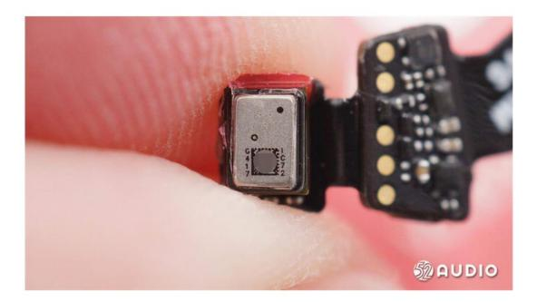
The bone conduction device VPU located on the small board is used to pick up the sound signal of the bone during a voice call to enhance the quality of the voice call.
