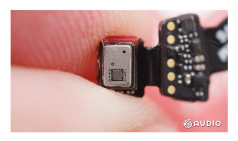
The bone conduction device VPU located on the small board is used to pick up the sound signal of the bone during a voice call to enhance the quality of the voice call.
