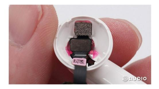
The circuit of the earbud module is connected to the earbud motherboard through the BTB connector. The bone conduction sensor is located directly above.
