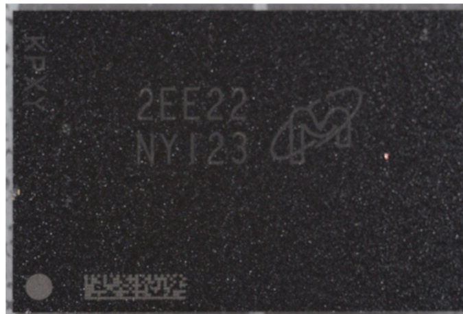
3D NAND Chip Extracted from Micron 3400 SSD with NVMe
