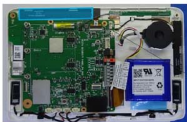
A first antenna (in blue) configured to provide operation in at least three frequency bands being used by 4G communication standards
