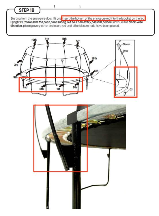
27. The Skywalker 16' Round Epic Series Trampoline includes a plurality of flexible enclosure rods, with each connected to the barrier net only at or near an upper peripheral part of the barrier net (red callout boxes added):
