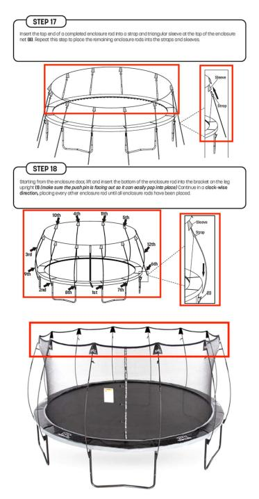
29. The flexible enclosure rods used in the Skywalker 16' Round Epic Series Trampoline are made of polyethylene-sleeved fiberglass (red callout boxes added):
