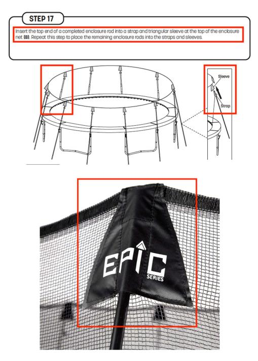
28. The Skywalker 16' Round Epic Series Trampoline includes a plurality of flexible enclosure rods, with each connected together at or toward the upper end of the flexible enclosure rods to draw the upper ends away from their natural rest state and towards the center of the mat (red callout boxes added):
