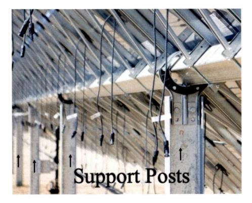
43. Defendant uses solar trackers that include a support frame, on which photovoltaic panels are rotatably mounted, that includes a torque tube beam which extends along the center for the frame. The torque tube beam is a central spine. The solar trackers being used by Defendant include transversely arranged elongated members to which the photovoltaic panels are mounted. The elongated members are panel carriers.
