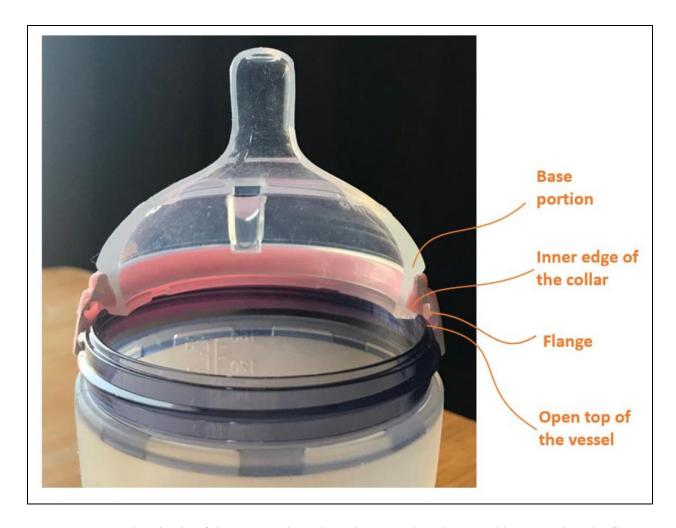
34. The nipple of the Accused Products is secured to the vessel by capturing the flange of the nipple between the collar and the open top of the vessel. For example, the image below demonstrates how the nipple secures to the vessel by capturing the nipple's flange between the exemplary pink collar and the open top of the vessel.
