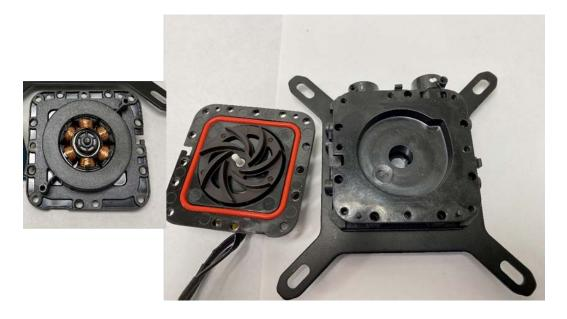
34. The Exemplary Infringing Products further include "a reservoir adapted to pass the cooling liquid therethrough." For example, as the image of the representative Lian Li Galahad product below shows, the Exemplary Infringing Products include a reservoir adapted to pass cooling liquid through it.
