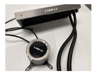
69. The Exemplary Infringing Products include "a set of four mounting legs configured to secure the heat-exchanging interface to a heat-generating component of a computer." For example, as the image of the representative Lian Li Galahad product below shows, the Exemplary Infringing Products include a set of four mounting legs configured to secure the heat-exchanging interface to a heat-generating component of a computer.
