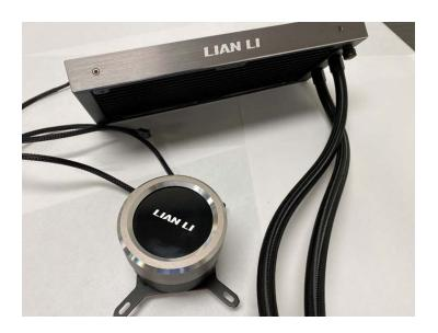
22. The Exemplary Infringing Products further include "a fan adapted to direct air to the heat radiator to dissipate heat from the cooling liquid to the surrounding atmosphere." For example, as the image of the representative Lian Li Galahad product below shows, the Exemplary Infringing Products include a fan that is adapted to direct air to the heat radiator to dissipate heat from the cooling liquid to the surrounding atmosphere.
