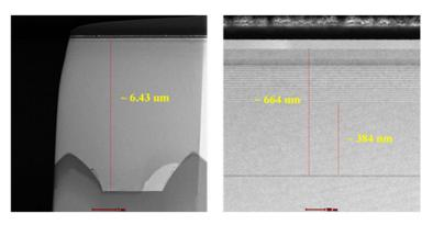
63. The layer structure in the image above right includes, in relevant part from bottom to top, an n-type semiconductor layer, a functional part, and a p-type semiconductor layer.
