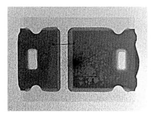
103. As the above images show, the LED package contains two metal lead frames spaced apart from each other. The optical image shows that each lead frame has a substantially flat top surface, a bottom surface, a fixing hole, and sidewalls between the top and bottom surfaces. LED chips are disposed on the top surface of the right lead frame in the optical image.
