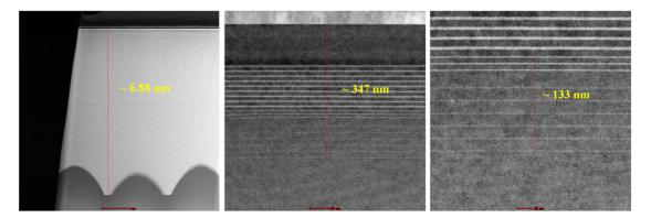
96. Based on the level of Indium doping in the active region, the superlattice layer, and the spacer layer, the spacer layer will have a bandgap smaller than the barrier layers of the multiquantum well, but higher than the bandgap of the quantum well layers.
