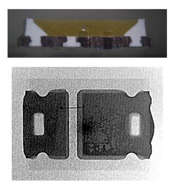
80. As the above images show, the LED package contains two lead frames spaced apart from each other. The optical microscope image show that each lead frames has an upper portion and a lower portion. Two LED chips are disposed on the upper portion of the right lead frame in
