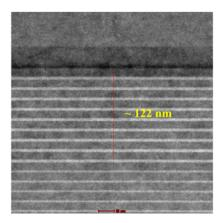
65. The above depicted functional part includes multiple active layers that include a multilayer stacked body including a plurality of thick film layers and a plurality of thin film layers alternately stacked in the direction. The thin film layers appear as relatively bright and thin layers (wells) separated by relatively thick dimmer layers (barriers). A multilayer stacked body can include, for example, a pair of wells and three surrounding barrier layers.
