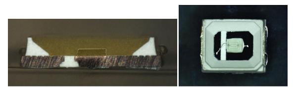
72. The above cross-sectional image also shows first (right) and second (left) lead frames that are spaced apart from each other. The cross-sectional also shows that at least part of
