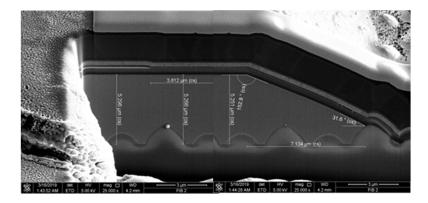
43. Upon information and belief, the method of fabricating a light emitting diode further comprises the step of forming a lower semiconductor layer, an active layer, and an upper semiconductor layer on the substrate. The resulting layers are shown in the scanning electron optical microscope image reproduced below.
