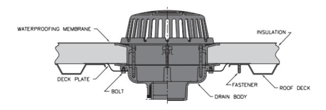
13. Zurn's Top-Set® roof drains include a novel combined drain support plate and under deck clamp assembly, which reduces the drain installation time and expense by eliminating a bottom installation of a drain and allowing installers to install the drain from the top.
