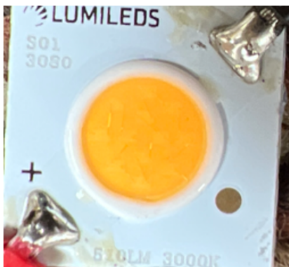
Figure 3A - 1 - LED Chip - Kichler C-Series LED Small Accent Light
