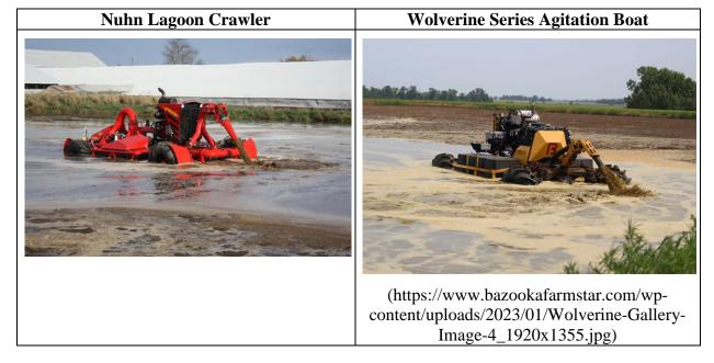
Atlas Ag has used and continues to use the submersible pump and the "Front Gun" of the Wolverine Series Agitation Boat to pump manure and return a percentage of the manure back to the pit or lagoon in the form of a high volume spray to disrupt a crust that can develop on the surface of a pit or lagoon and recirculate the manure as shown below:
