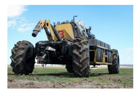
28. The Wolverine Series Agitation Boat also includes a fluid nozzle connected to a pump. The pump is powered by an engine. The Wolverine Series Agitation Boat is described as having an "18" Bazooka Farmstar Submersible Pump & Front Gun." (https://www.bazookafarmstar.com/equipment/wolverine-agitation-boat/#pid=4)
