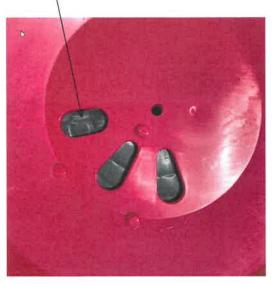
When the shut-off adjustment plate is moved to the <u>fully open position</u> the three exit openings in the shut-off adjustment plate are aligned with the three openings in the hopper:
