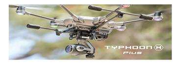
Capturing breathtaking still photos and 4K videos is made easy with the Yuneec Typhoon H Plus drone. Its Intel RealSense Technology detects and avoids obstacles while navigating safely through its set route or toward you with the Follow Me mode. The ST16S all-in-one controller has a large 7-inch screen that displays the real-time footage from the camera.
