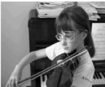
Figure 6.6 QCF frame with highlighted macroblock
