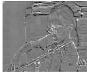
Figure 6.8 Residual after subtracting intra prediction
