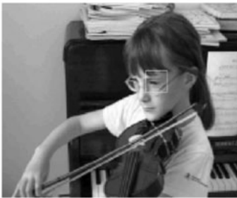
Figure 6.6 QCFI frame with highlighted macroblock
