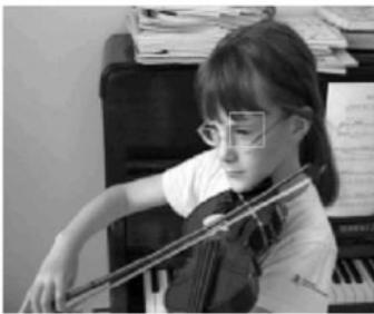
Figure 6.6 QCIF frame with highlighted macroblock
