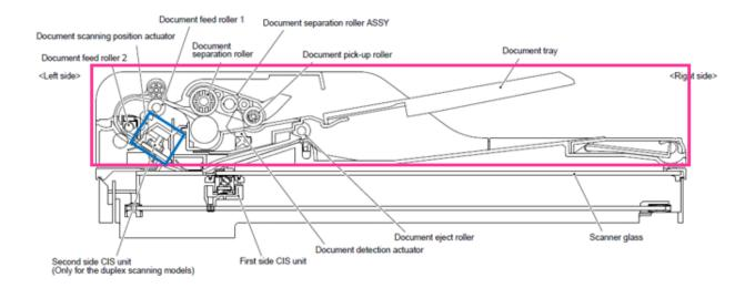
20. The claimed second reading portion of the MFC-L3770CDW is housed in the flatbed scanner. Within the flatbed scanner, a CIS unit contains a second light source, a lamp, that emits light onto the other, downward-facing side of the document to read that surface.
