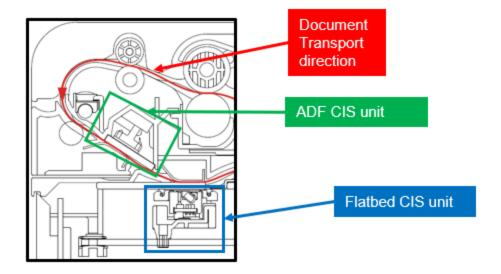
22. Both CIS units shut off simultaneously after the document has passed through the reading region of the flatbed CIS unit, and thus the ADF CIS unit is turned off after the document has passed through the flatbed scanner.
