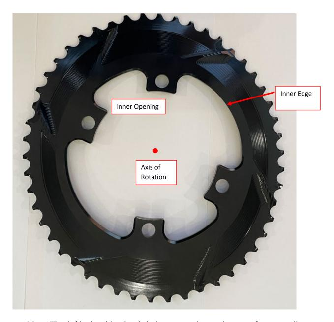
15. The infringing bicycle chainrings comprise an inner surface extending between the inner edge and an outer edge where a plurality of chain ring teeth emanate.
