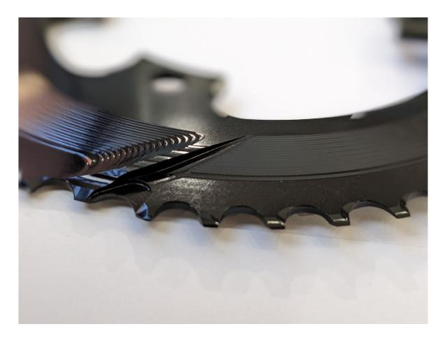
20. These ramps on the absoluteBLACK chainrings are configured with a lifting surface to concurrently engage at least one link of a bicycle chain at two or more distinct pivot points along the length of the chain link to initiate stable lift of the bicycle chain without assistance from any of the plurality of chain ring teeth as recited in the asserted patent claims.
