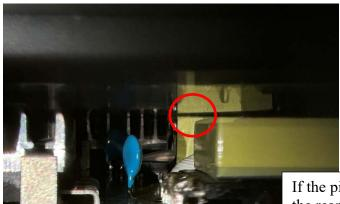
If the pin is removed from the power source board, the rear cover contacts with the circuit element when the rear cover is pushed.
