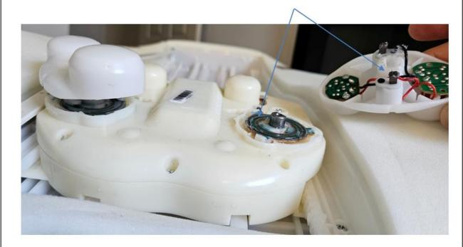
24. The conductive brushes are mounted to the substrate and connected to a heater mounted to the substrate. Each of the conductive brushes is in engagement with one of the annular contacts for maintaining engagement during rotation of the substrate relative to the housing.
