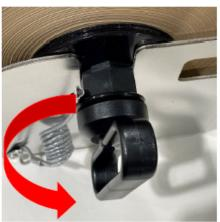
If the paper is tearing when pulled, then tension must be decreased. Rotate the Adjustment Handle COUNTERCLOCKWISE.
