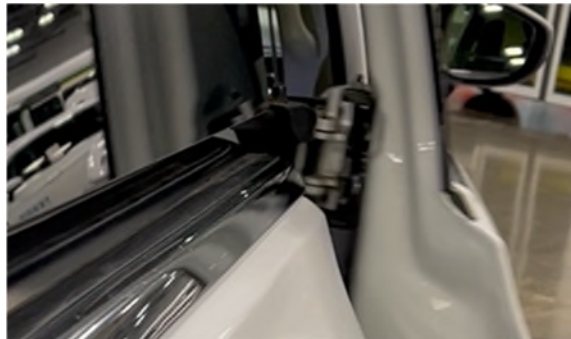
Collapsed condition at first end upon full closure of door
