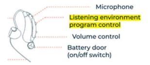
36. As explained on page 32 of Exhibit D, the "listening environment program control" button on the hearing aid is a switching device which, when pressed, "change[s] the listening environment." Pressing the button causes the processor to cease execution of one of the programmed listening environments and commence execution of another programmed listening environments.
