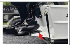
The picture to the left shows the Defendant's outboard jet motor intake angled at an upward slope.
