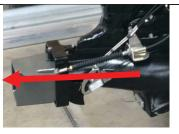
As pictured, the steering nozzle receives water flow from the jet by way of the conduit.
