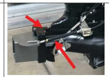
This element is infringed, as pictured to the left, as Defendant's product is capable of rotating its outer frame and steering nozzle relative to the conduit along an axis defined by the first pair of axles. Defendant's product even has the steering element identical to the patent figure pasted above.
