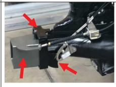
Defendant uses an outer frame to join the conduit and steering nozzle – as pictured and as shown in the patent figure above.
